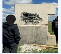
Using the results from these tests, the KarabloK units are proven to be compliant with STANAG 2280, the NATO standard for ballistic, blast and impact barriers.
